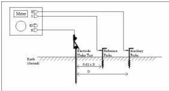
Figure 3: Single Electrode Measurement Setup
