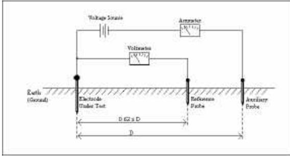
Figure 2: Single Electrode Measuring Method
