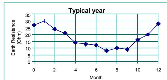
Figure 9: Typical electrode resistance to remote earth in a year
