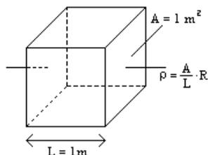
Figure 7: Soil Resistivity Definition Cube
