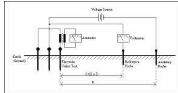
Figure 5: Multiple Electrode Measuring Method
