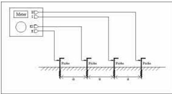
Figure 11: Soil Resistivity – Four Pole Setup
